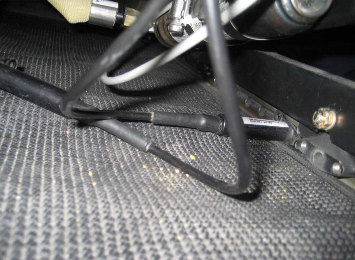
**Cessna 172S, Loosened Seat Lock Attach Screws, ATA 2510**
